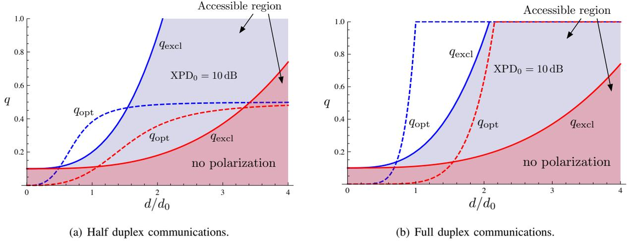
**Fig. 3:** Accessible and optimal terminal probabilities of transmission as a function of  $d/d_0$  and for  $\varepsilon = 0.1$ . In both cases, two polarization strategies are considered: (i) no polarization (drawn in red) and (ii) polarization with  $\text{XPDP}_0 = 10$  dB (drawn in blue).
