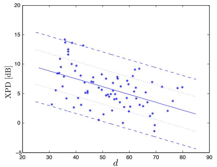
**Fig. 8:** XPD (logarithmic scale) in the outdoor-to-indoor scenario.
