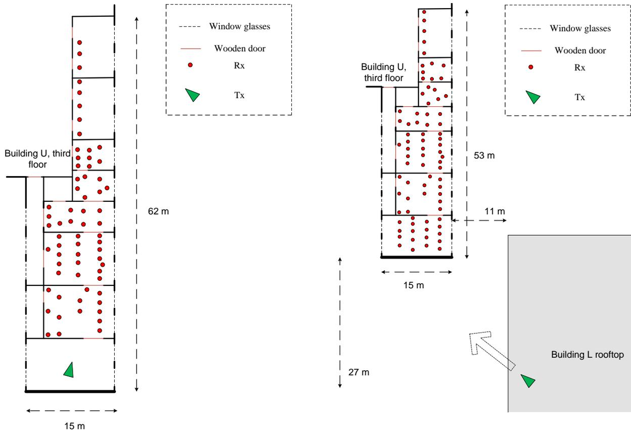
(a) Indoor-to-indoor measurement setup.
