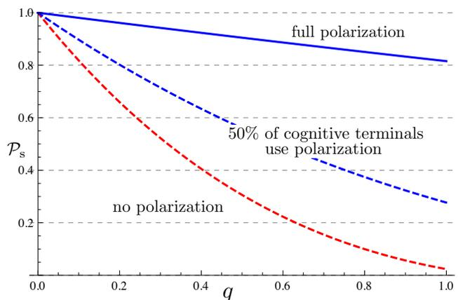
(b) Link probability of outage on the primary network as a function of the probability of transmission.
