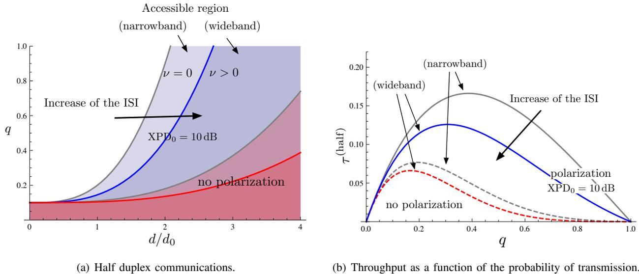
**Fig. 13:** Impact of the channel fading on the system-level performance. The parameter value  $\nu = 0$  and  $\nu > 0$  correspond to narrowband scenarios and wideband scenario, respectively.
