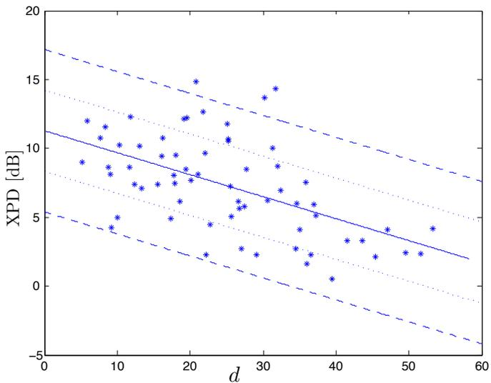
**Fig. 5:** XPD in logarithmic scale, as a function of the Tx distance, in the indoor-to-indoor scenario with an initial horizontal polarization.
