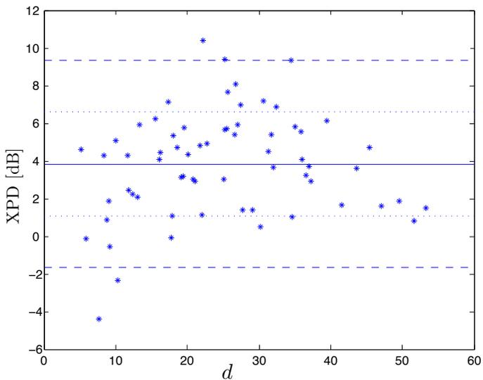
**Fig. 7:** XPD in logarithmic scale, as a function of the Tx distance, in the indoor-to-indoor scenario with an initial vertical polarization.
