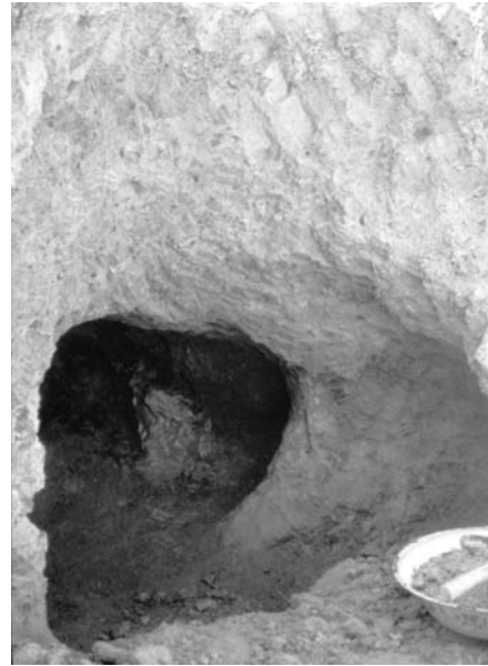
Figure 5. Gallery extraction is favoured among the Bissa potters of Luanda (Burkina Faso). As the superficial layer is considered inadequate for pottery making, clay is exploited in galleries below it (Photo A. Livingstone Smith).
