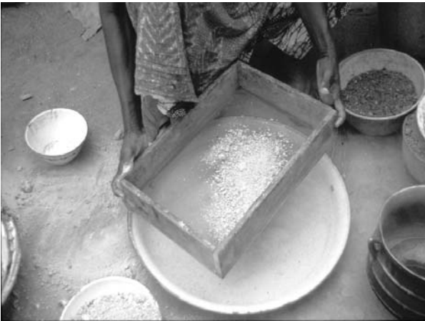
Figure 11. Sieving the pounded raw material with an imported nylon mesh among the Ewe of Kpalime, Southern Togo (Photo A. Livingstone Smith).
