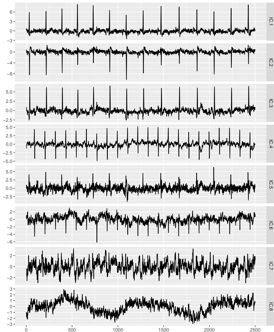
Figure 3: Independent components based on JADE for the ECG measurements of the pregnant women dataset.
