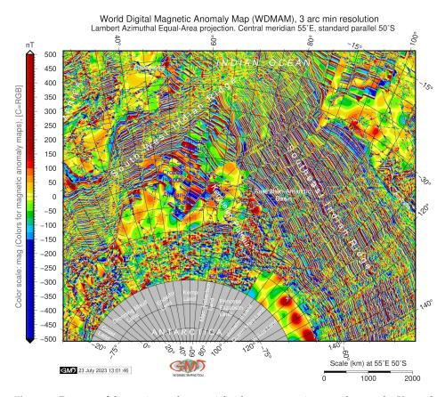
**Figure 9.** Patterns of the marine and terrestrial airborne magnetic anomaly over the Kerguelen Plateau on a three-minute resolution grid of WDMAM, south-west Indian Ocean. Map source: author.
