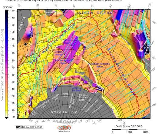
**Figure 4.** Spreading half rates of the ocean crust over the Kerguelen Plateau region, east Antarctic and south-west Indian Ocean with added GSFML data. Mapping tool: GMT. Map source: author.
