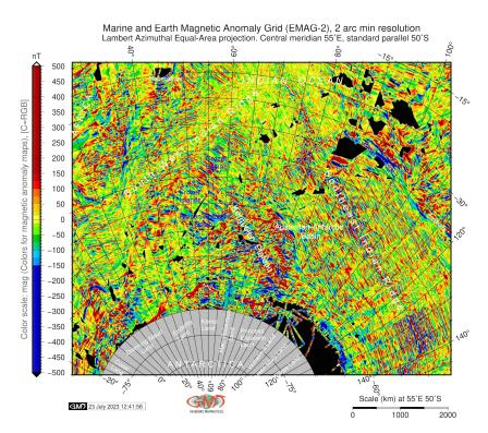
**Figure 10.** Marine and Earth airborne magnetic anomaly grid based on EMAG-2 over the Kerguelen Plateau region. Black areas signify "no data" in the original grid. Map source: author.
