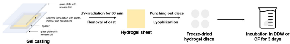
Figure 1. Schematic representation of the production of hydrogel sheets via gel casting, followed by punching out of circular samples, lyophilization and start of the swelling experiments.
