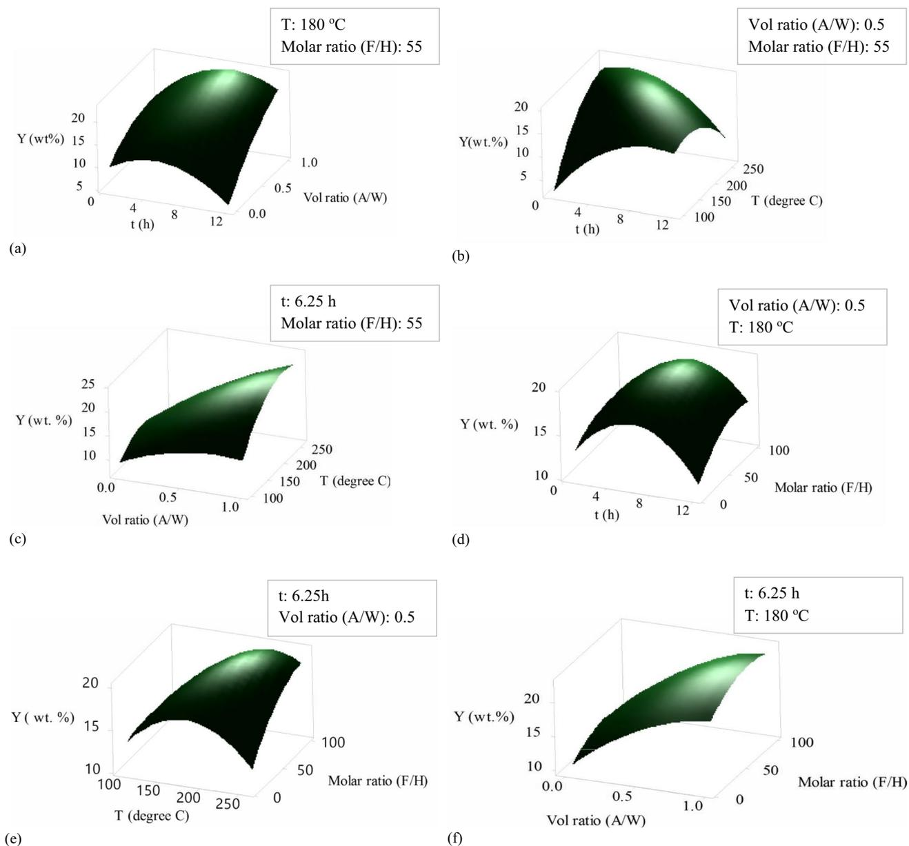
**Fig. 3** Combined effects of the process variables on the oil yield. Values of the process variables held constant are presented in legends. Herein,  $t$ ,  $T$ , vol ratio (A/W), and molar ratio (F/H) denote time (h), temperature ( $^{\circ}\text{C}$ ), alcohol/water v/v ratio, and  $\text{Fe}^{3+}/\text{H}_2\text{O}_2$  molar ratio respectively
