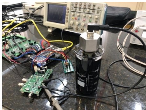
Fig. 6. Calibration setup for the capacitive sensor (immersed in the sample).
