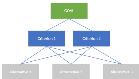
Figure 2 - One-Level Analytic Hierarchy Process with three alternatives
