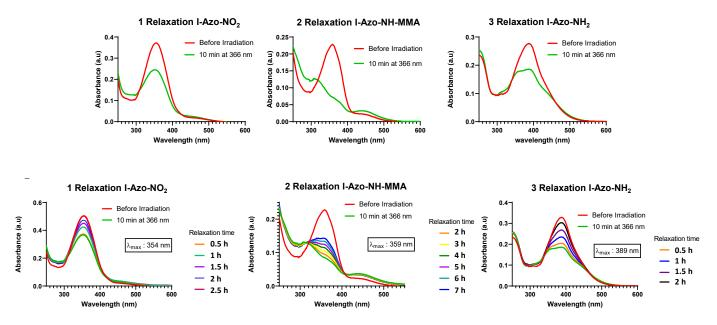
**Figure 5.** UV-Vis spectra for I–azo–NO<sub>2</sub> (**A1**), I-azo-NH-MMA (**A2**) and I–azo–NH<sub>2</sub> (**A3**) before (red) and after (green) a 10 min exposure to 366 nm light. Thermal relaxation spectra in the dark for I–azo–NO<sub>2</sub> (**B1**), I–azo–NH–MMA (**B2**) and I–azo–NH2 (**B3**).
