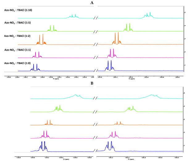
**Figure 4.** Stack plot of <sup>19</sup>F-NMR spectra of I–azo–NO2 and I-azo-NH-MMA (CDCl<sub>3</sub>), at different molar ratios of I-azo-NO<sub>2</sub>/TBACl (**A**) and I-azo-NH-MMA/TBACl (**B**). Molar ratios: a) 1:0; b) 1:1; c) 1:2; d) 1:5; e) 1:10.
