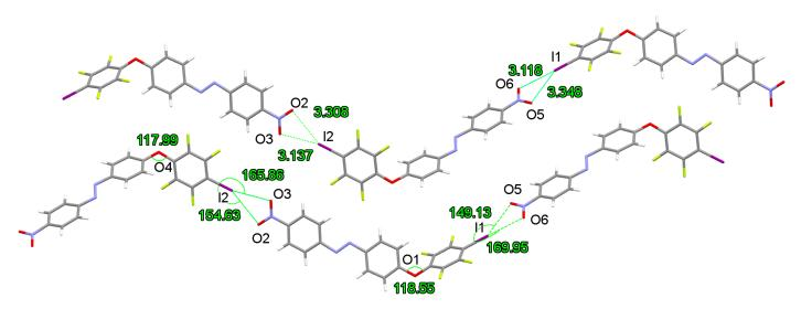
**Figure 1.** X-ray structure of I–azo–NO<sub>2</sub> developing undulating parallel chains due to two O…I halogen bonds. Colors are as follows: grey, C; blue, N; red, O; white, H; yellow, F; purple, I. O…I bond distances (Å) and C-I…O bond angles (°).
