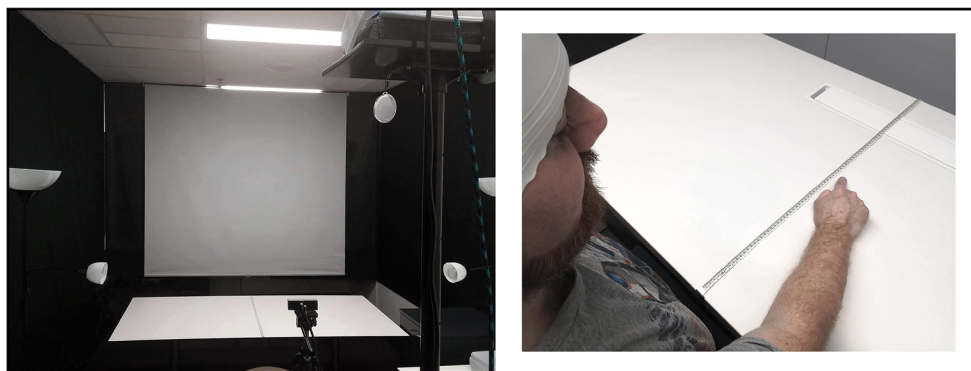
Fig. 5 Setup 3D-HDtDCS lab. The participant sat on a stool behind a table located in the middle of the room (~200 cm behind the projection screen). The projector is seen ~400 cm in front of the screen behind the cameras. In front of the stool, a measuring tape is visible that counted out from the participant towards the screen (see right panel). On the
