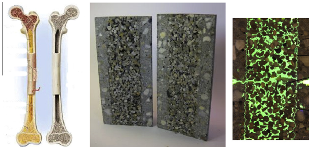
Fig. 5. Porous concrete healing similar to spongy bone filled with epoxy, after Sangadji and Schlangen (2012).
