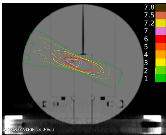
Fig. 3. Visualisation of isodoses in the coronal plane XZ passing the isocentre for the 16 mm collimator. The dose depth profile was defined along the axis, which passes by the isocentre and the dose maximum point. The depth dose profile orientation was adapted to each collimator size as the spatial positions of the sources depends on the collimator.
