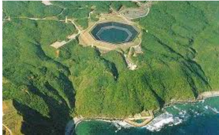
Figure 2.3: Seawater-based pumped storage plant in Okinawa, Japan.
