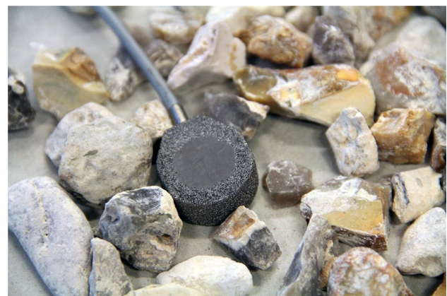
Fig. 3 Picture of the new generation of embedded piezoelectric transducers
