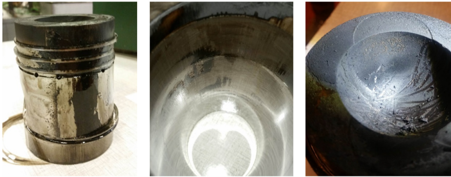
Figure 34: Left: Black trace on the side of the piston. Middle: Vertical scratches in the cylinder. Right: Cylinder head with black and green deposits.
