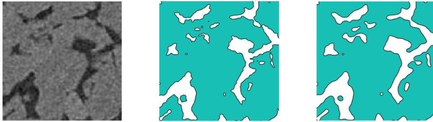
Figure 5.3: Comparison between : (a) a slice of the micro-CT scan, (b) thresholding process obtained by Otsu's method at 76 grayscale value, (c) level-set segmentation
