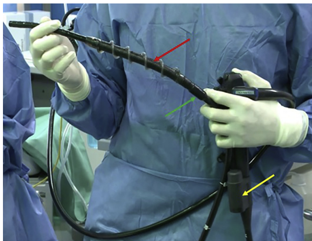
Figure 1. Motorized Spiral Enteroscope PSF-1 (PowerSpiral; Olympus Medical Systems Corporation, Tokyo, Japan) is a reusable endoscope, similar to a pediatric colonoscope of 1680 mm in length, with an outer diameter of 11.3 mm at the insertion portion. An integrated electric motor is used to rotate a short disposable spiral overtube ( red arrow , 240 mm length, 31.1 mm outer diameter of the soft spiral fins) that is attached to a rotation coupler ( green arrow ) located 40 cm proximal to the endoscope's tip. Direction and speed of motorized rotation of the spiral section is controlled by a foot pedal switch (not shown). Clockwise and counterclockwise rotation is used to traverse the small bowel by "pleating" or "unpleating" the small bowel onto or from the insertion tube, respectively. The direction and force that is applied to the tissue by spiral rotation is continuously monitored by the system and shown on the display (spiral rotation force indicator, see Fig. 2A and C). An integrated safety mechanism stops spiral rotation automatically if a certain threshold is exceeded.
