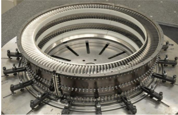
Figure 1-11. Finalised composite booster (standing on a clamping tool). Courtesy of Safran Aero Boosters.
