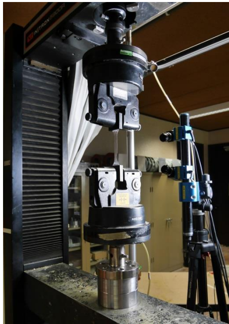
Figure G-8. Steel sheet specimen mounted on the test bench for quasi-static uniaxial tensile testing with strain monitoring by digital image correlation. The pair of cameras is visible at right of the picture, while the light source used for correct illumination of the specimen speckle pattern is even further to the right, out of the picture frame.
