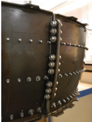
Figure 1-5. Close-up view of two half composite casings bolted together at the axial flanges.
