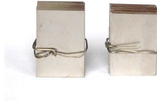
Figure G-3. (a) Controlled temperature program applied for the measurement of the steel sheet CTE by TMA (heating & cooling rates: 2 °C/min), (b) samples prepared in the form of bundles of rectangular pieces of steel sheet (one sample by reference direction).
