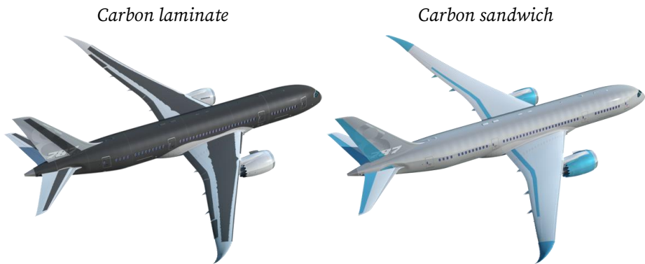
Figure 1-1. Distribution of carbon laminate (left) and carbon sandwich (right) composites in the Boeing 787' structure [15]
