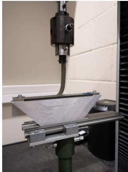
Figure 6-6. Peel test specimen being peeled off at 90° with the fixed arm peel test apparatus mounted on the test bench of a universal testing machine.
