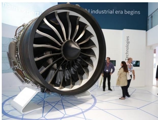
Figure 1-2. General Electric GENx engine with carbon fibre composite fan blades and fan case. Visitors set the scale. [21]
