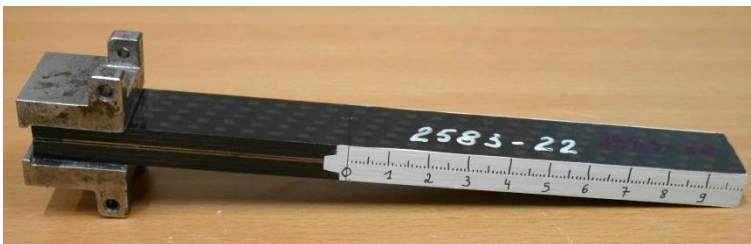
Figure 6-5. Beam-type LEFM test specimen prepared for the DCB test.
