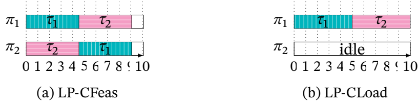
Figure 5.4: Rectangle schedule computed from LP-CFeas versus schedule favouring fast cores utilisation computed from LP-CLoad
