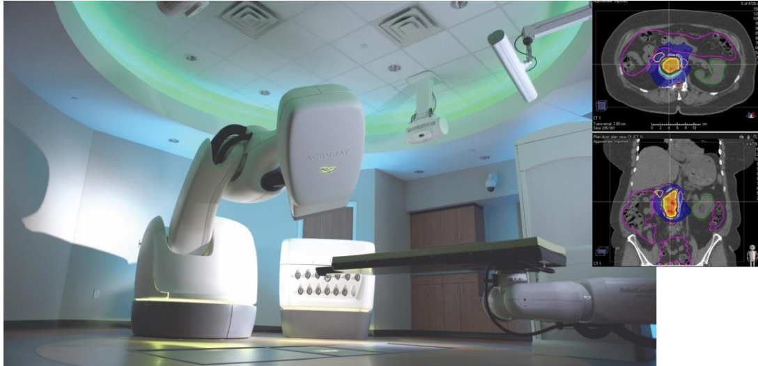
Figure 11. View of the Cyberknife M6 system, with the robotic treatment head and couch, and the dose images for a stereotactic treatment on the right (small target in the abdomen). Source: https://delraynewspaper.com/wp-content/uploads/2018/07/cyberknife.jpeg
