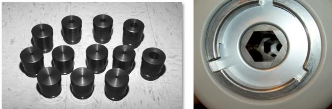
Figure 29. Left: the 12 fixed circular collimators, with their diameter at isocenter varying from 5 to 60 mm. Right: view from under the iris collimator, showing the two banks of tungsten segments rotated with respect to each other.
