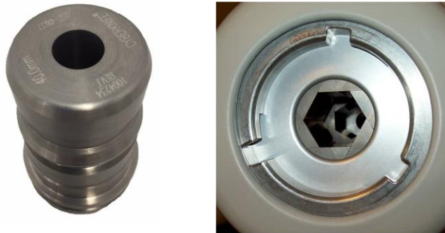
Figure 17. Left : fixed 40 mm collimator. The actual collimator opening is close to 20 mm as it is placed at approximately 40 cm from the source, thus forming a 40 mm beam size at 80 cm distance. Right: view of the iris collimator from below the treatment head. The two banks of leaves can be seen ( https://www.slideshare.net/JustinVinci/cyberknife-at-saint-raphaels-campusrevb ).
