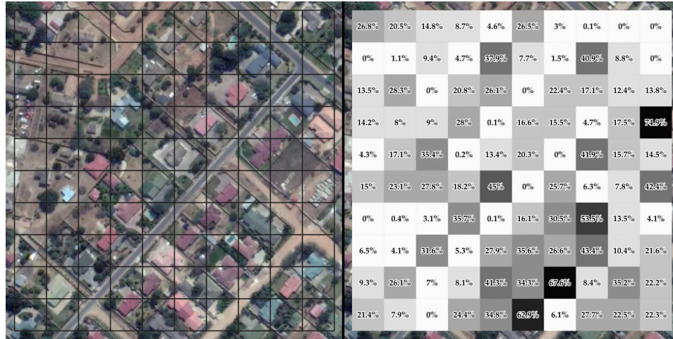
Figure 4.3: Percentage of Built-Up Areas per 30 m pixel in a suburban area of Lusaka, Zambia.
