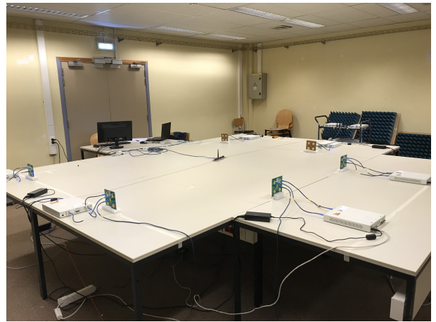
Fig. 3. The full setup consists of 6 independent anchors, all connected to a central computer. The emitter antenna is a 2.4GHz monopole mounted on a movable stand.
