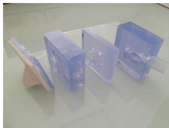
Figure 32. Illustration of the nasal cast used for the assessment of the drug distribution in the nasal cavity (Aptar© Pharma)
