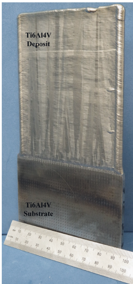
FIGURE 6: Ti6Al4V wall structure built with a BH of 105 mm on a 3 mm thick Ti6Al4V substrate using a wire-fed EBAM process in a vacuum environment.
