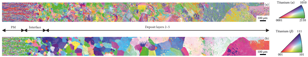
FIGURE 10: EBSD map of (a) the \alpha phase and (b) numerical reconstruction of the parent \beta phase in the Ti6Al4V wall structure built on a Ti6Al4V substrate using wire-fed EBAM.
