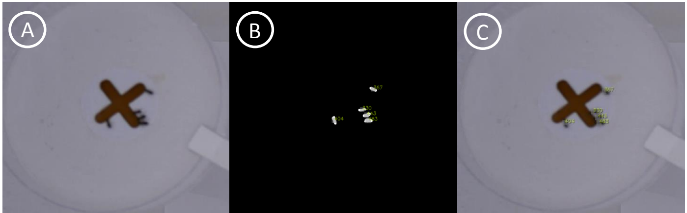
Figure S1. Ants of L. niger feeding at a food source are automatically detected by USETracker software. A Input frame. B Processing frame. C Output frame.
