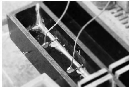
(b) Zoom on the embedded transducers
