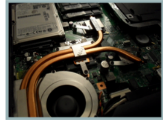
Figure 1.5: Electronic cooling systems are normally Copper/Water HP.
