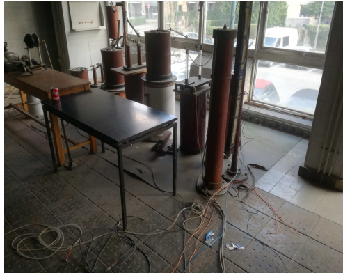
FIGURE D.5: Lightning impulse generator used in the laboratory tests.
