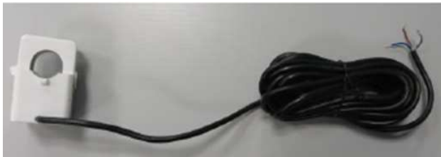
FIGURE C.2: Current measurement CT used by the TFS system.
