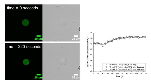
**Fig. S8** Fluorescence and bright-field microscopy images before (top) and after (bottom) addition of NaCl to GUVs previously incubated with LUVs (10 mol % transporter).  $CP_4K_4$  is excluded from GUVs. The normalized fluorescence intensity over time is given for individual GUVs from independent experiments.
