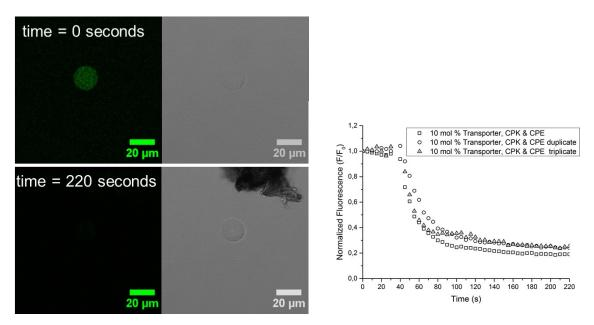
**Fig. S6** Fluorescence and bright-field microscopy images before (top) and after (bottom) addition of NaCl to GUVs previously incubated with LUVs (10 mol % transporter). The normalized fluorescence intensity over time is given for individual GUVs from independent experiments.
