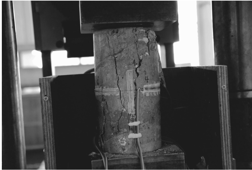
Figure 6. Failure mechanism of the cylinder. The failure mode is a mixed mode between splitting and shear failure
