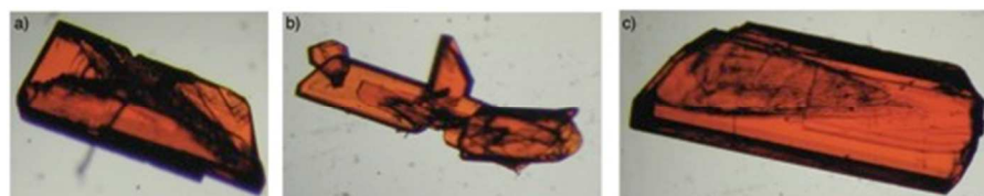
Figure 17. Optical microscopy images of the single crystals obtained from the trimeric complex between TANP and (a) 4-chlorophenylboronic acid 10 , (b) 4-bromophenylboronic acid 11 and (c) when an equal molar solution of 4-chloro and 4-bromophenylboronic acid was used.
