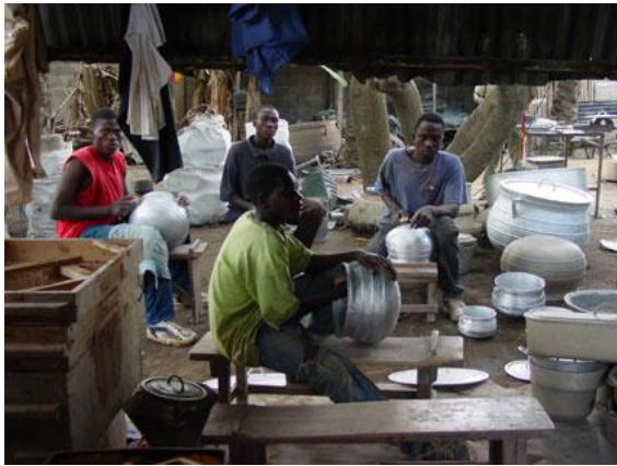
Figure III.2-7 Phase de finition atelier SMOAC
