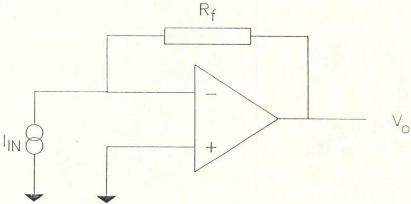
Figure 12: The current to voltage converter.
