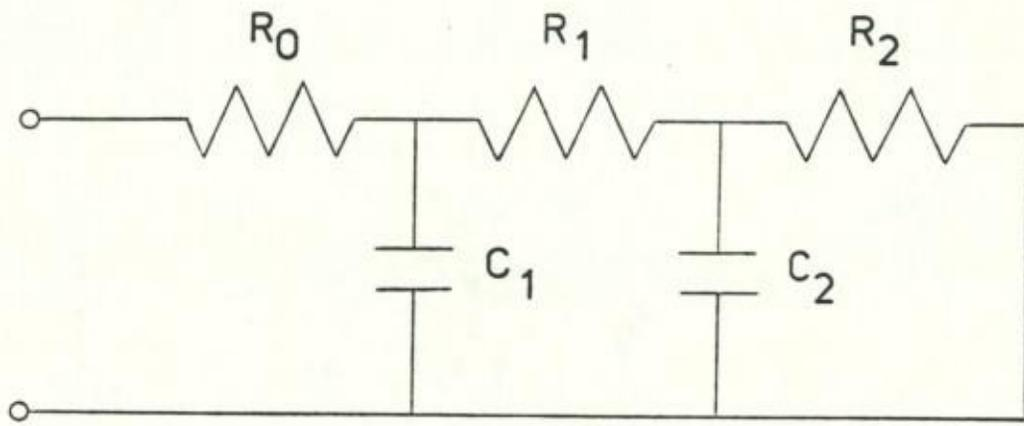
Figure 18: Electrical equivalent circuit used to fit the operational impedance spectrum of a two time-constant system.
