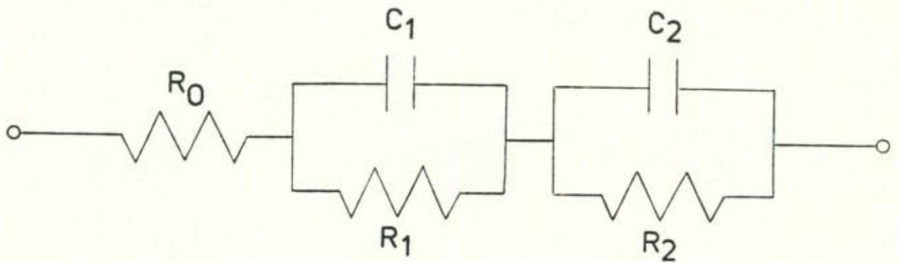
Figure 19: Electrical equivalent circuit of a plant cell consisting of a plasmalemma and tonoplast in series.
