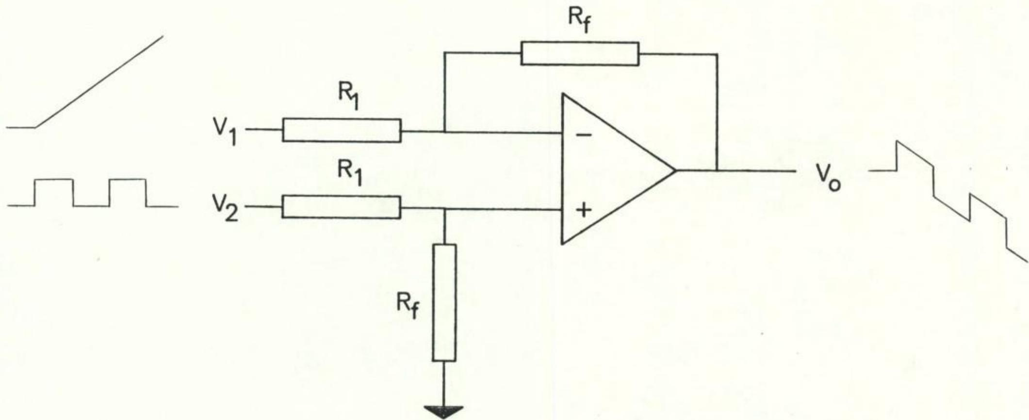
Figure 11: The differential amplifier.
