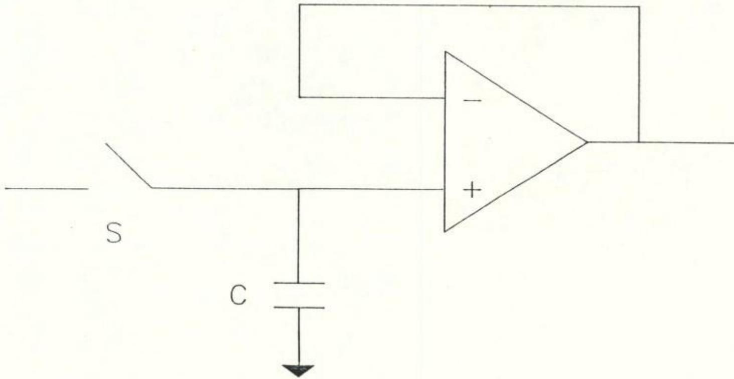
Figure 13: The sample-and-hold circuit.
