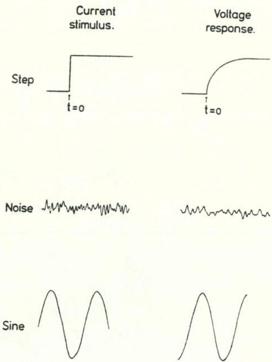
Figure 6: Electrical signals used for the impedance spectroscopy.
