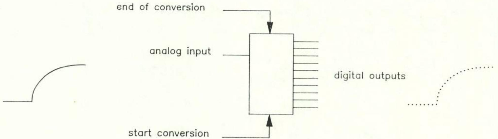
Figure 14: The analog to digital converter.
