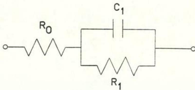
Figure 17: The simplest electrical equivalent circuit of a plant cell.
