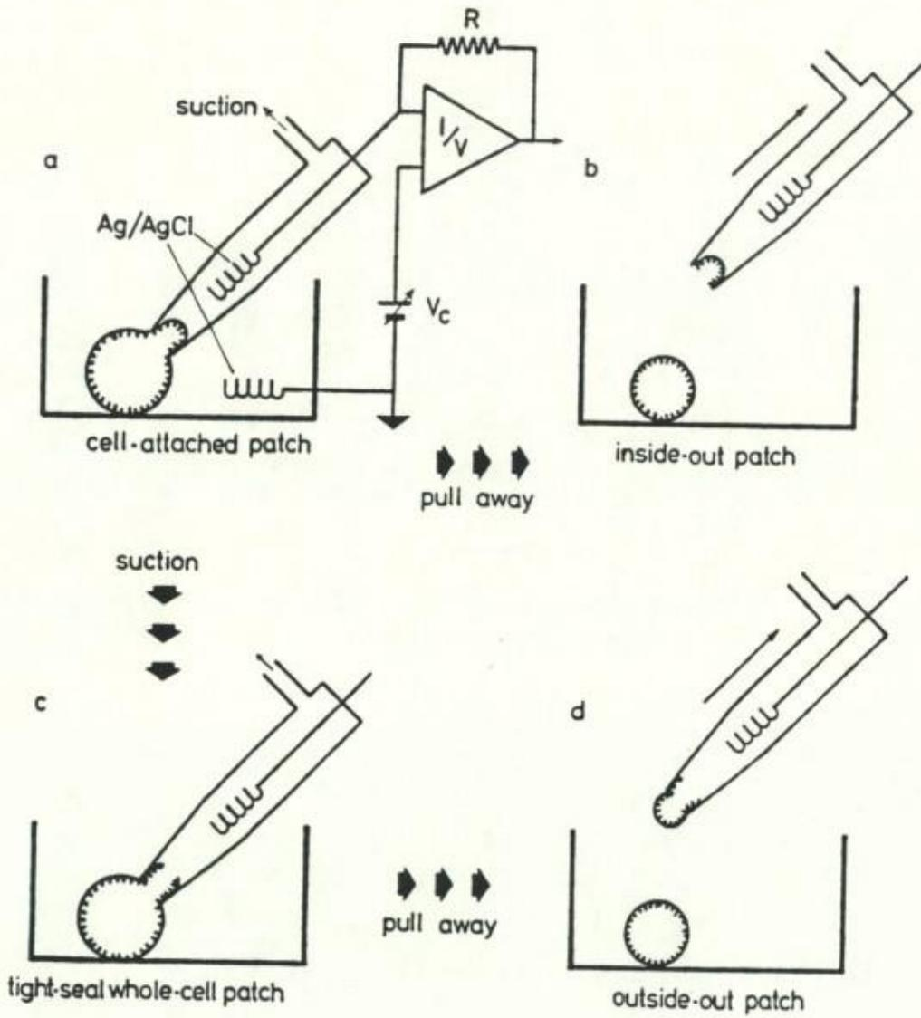
Figure 27: Schematic diagram of the procedure used for patch-clamp techniques.  $I/V$ : high gain low input noise current to voltage converter;  $V_c$ : voltage command; Ag/AgCl: silver chlorided electrodes.
