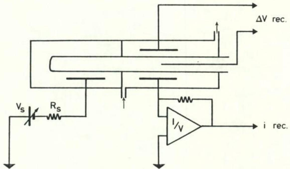
Figure 7: Schematic diagram of a simple current clamp device.
