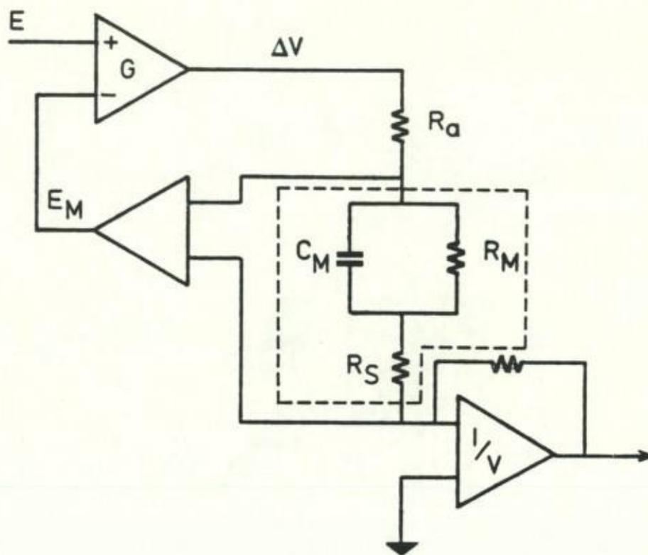
Figure 8: Schematic diagram of a voltage clamp device.
