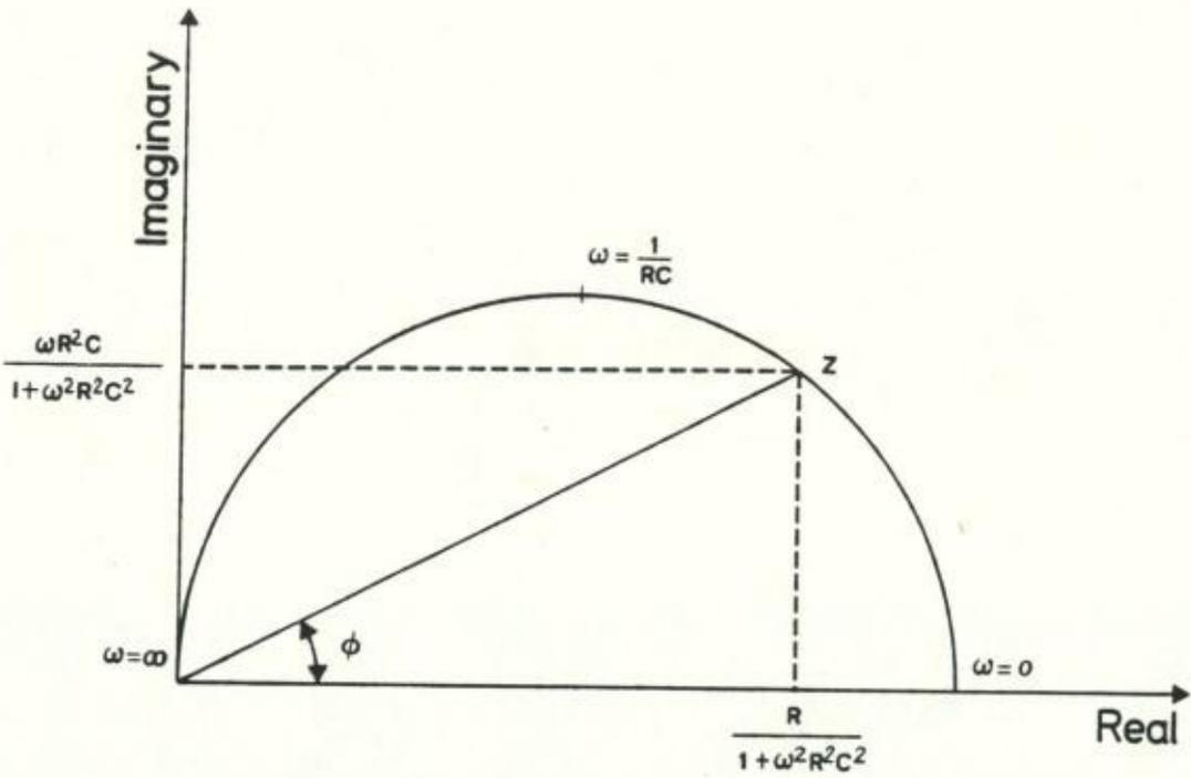
Figure 16: Impedance locus diagram for the parallel resistor-capacitor circuit
