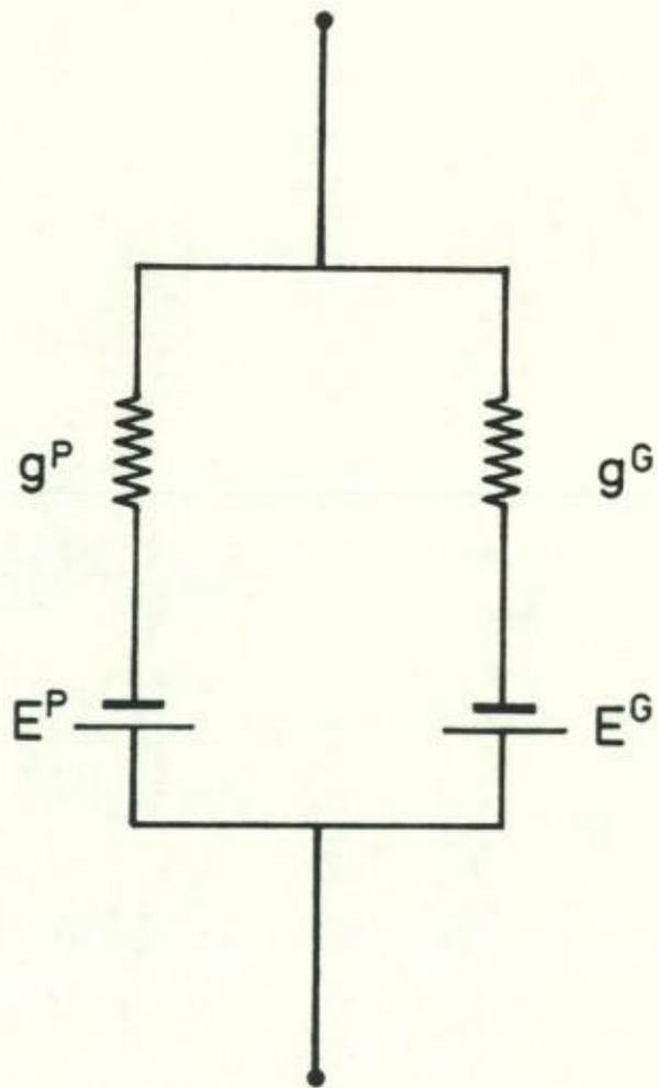
Figure 3: Electrical equivalent circuit for a membrane containing electrogenic ion pump.
