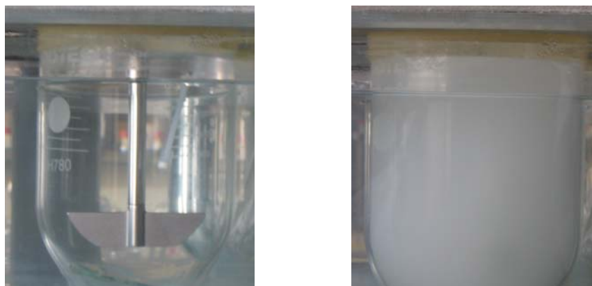
Figure IV 6 3. Photograph of dissolution baths - before (pH 1.3) and following (pH 6.3) drug reprecipitation.
