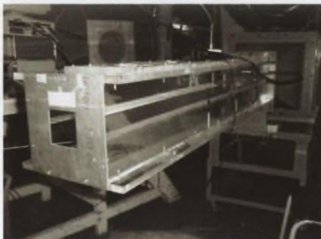
FIGURE B.3 – The square blockage installed on the test section of the wind-tunnel.
