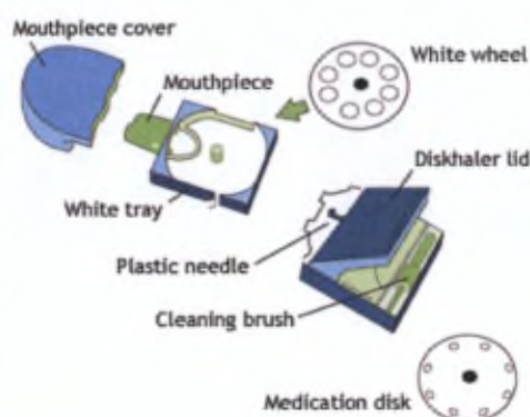
Figure 11: Schematic presentation of the Diskhaler ® (Asthma, 2008)
