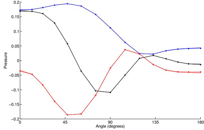
**Fig. 3.28.** Infinitesimal cylinder radiation with a second order enrichment at 500 Hz with a uniform mean flow  $\mathbf{v}_0 = -85m/s \mathbf{1}z$ ,  $n_p = 12$ ,  $n_r = 12$ : illustration of the analytical and the computed pressure along the interface  $\Gamma$ : absolute (blue), real (red) and imaginary (black) part of the pressure.
