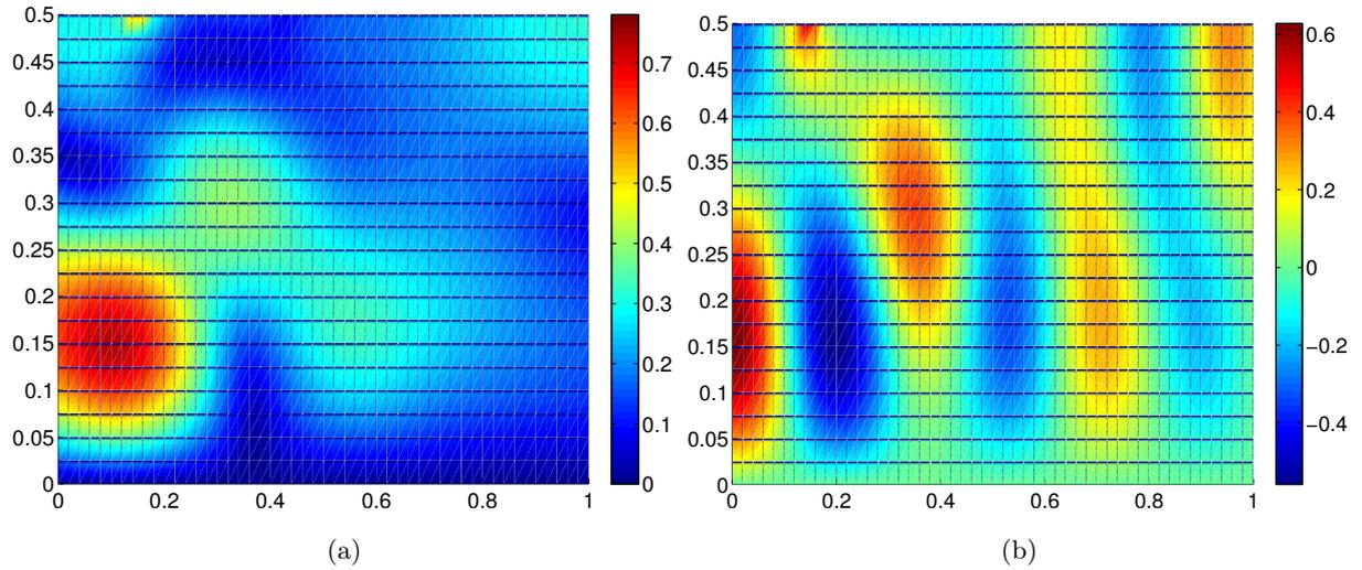
**Fig. 3.14.** ACTRAN<sup>TM</sup> results for the convected ( $\mathbf{v}_0 = -100m/s\mathbf{1}_z$ ) propagation at 800 Hz of the second mode of the first azimuthal order in a lined duct: (a) Absolute part of the acoustic pressure (b) Real part of the acoustic pressure.
