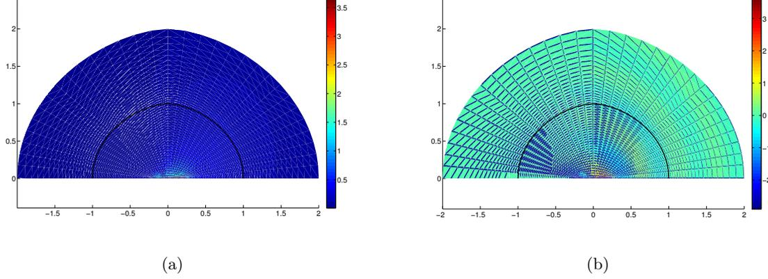
**Fig. 3.26.** Computed results for the infinitesimal cylinder radiation at 500 Hz with a uniform mean flow  $\mathbf{v}_0 = -85m/s \mathbf{1}_z$ : (a) Absolute part of the acoustic pressure (b) Real part of the acoustic pressure
