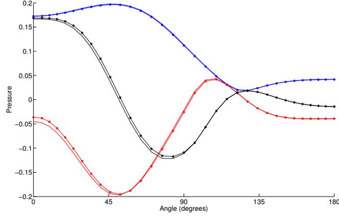
**Fig. 3.27.** Infinitesimal cylinder radiation with a constant enrichment at 500 Hz with a uniform mean flow  $\mathbf{v}_0 = -85m/s \mathbf{1}_z$ ,  $n_p = 30$ ,  $n_r = 30$ : illustration of the analytical and the computed pressure along the interface  $\Gamma$ : absolute (blue), real (red) and imaginary (black) part of the pressure.
