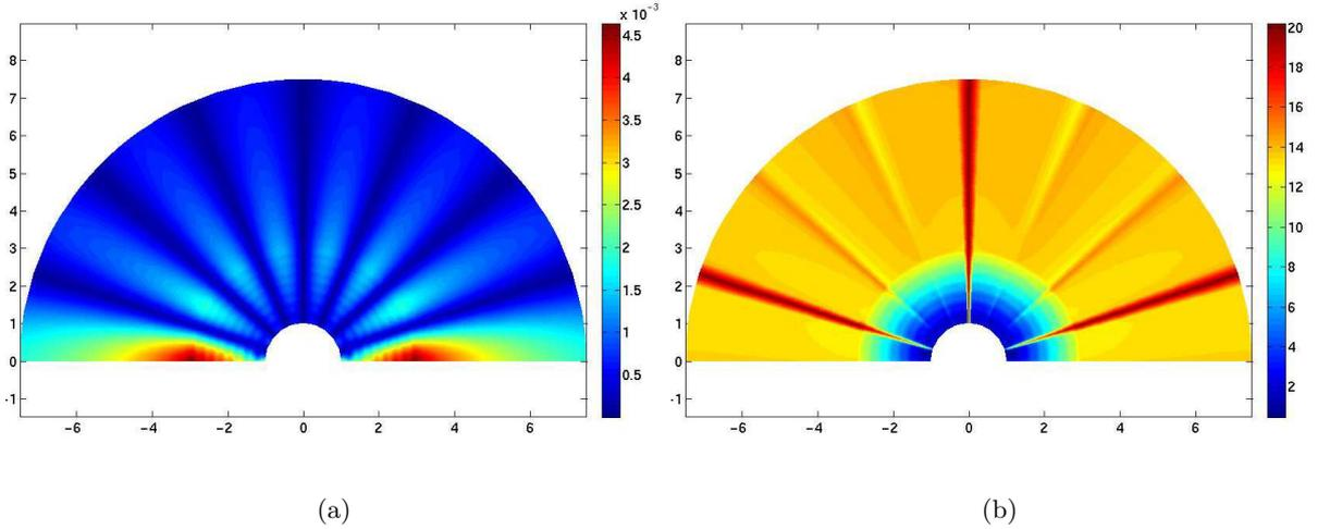
**Fig. 3.22.** Multipole ( $N = 7$ ) radiation: MIPUM 0 2 1 (a) Discrete  $L^2$  norm (b) Relative discrete  $L^2$  norm [%]: ( $700\text{Hz}$ ,  $kr_S = 12.94$ ), number of elements in the radial direction:  $n_r = 70$ , and in the circumferential one:  $n_\theta = 70$ .
