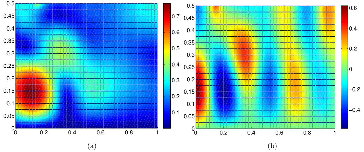
**Fig. 3.13.** MIPUM 0 computed results for the convected ( $\mathbf{v}_0 = -100m/s\mathbf{1}_z$ ) propagation at 800 Hz of the second mode of the first azimuthal order in a lined duct: (a) Absolute part of the acoustic pressure (b) Real part of the acoustic pressure.
