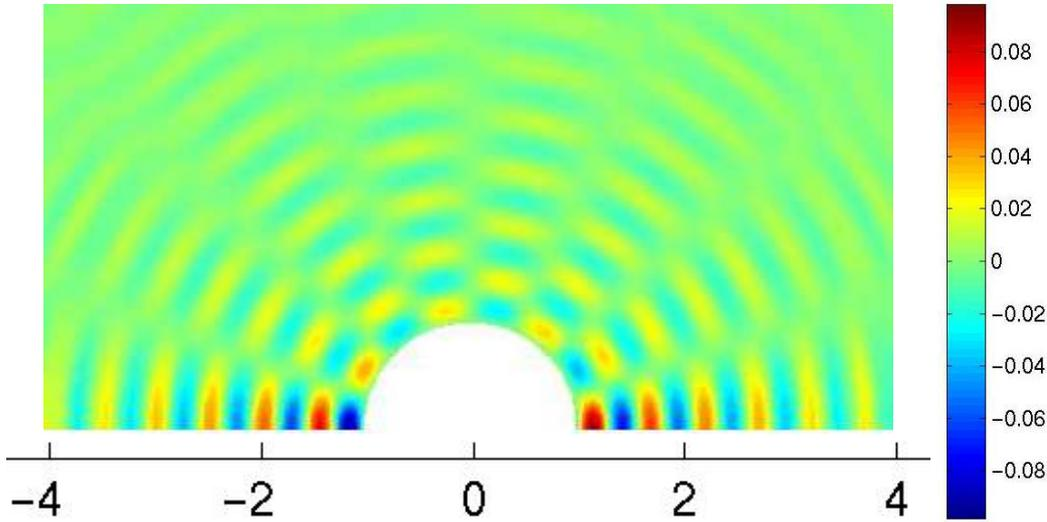
**Fig. 3.20.** Multipole ( $N = 7$ ) radiation: real part of the MIPUM 0 2 1 computed pressure ( $700Hz$ ,  $kr_S = 12.94$ ), number of elements in the radial direction:  $n_r = 70$ , and in the circumferential one:  $n_\theta = 70$ .
