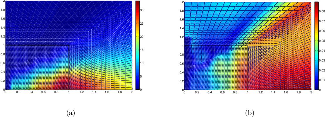
**Fig. 3.24.** MIPUM 0-4-1 computed results for the radiation of a rigid piston in an infinite domain at 500Hz: (a) Discrete  $L^2$  norm (b) Relative discrete  $L^2$  norm.
