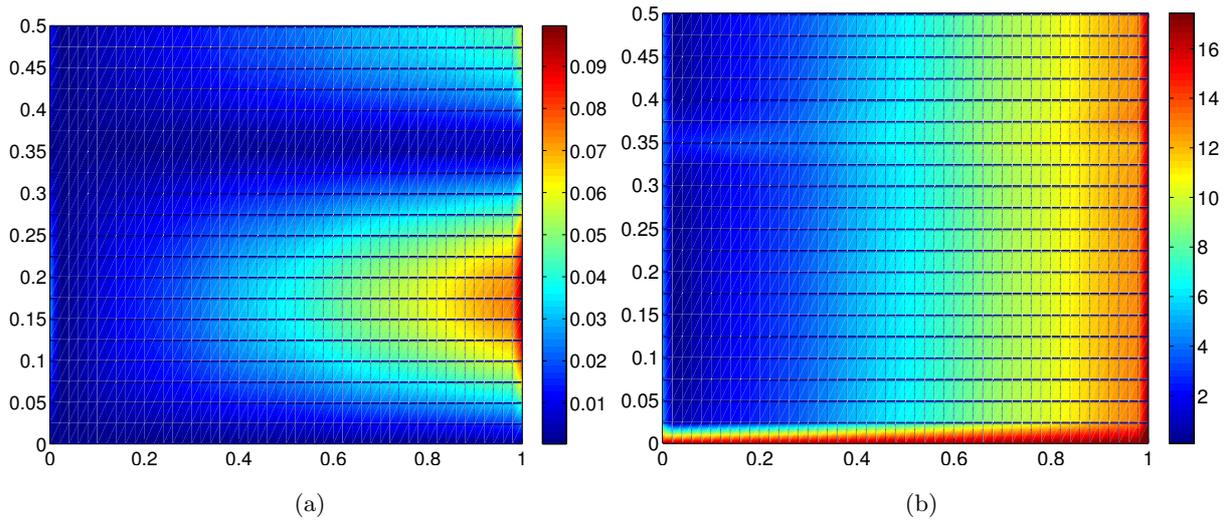
**Fig. 3.12.** Convected ( $\mathbf{v}_0 = -100m/s\mathbf{1}_z$ ) propagation at 800 Hz of the second mode of the first azimuthal order in a hard walled duct: MIPUM 0 (a) Discrete  $L^2$  norm (b) Relative discrete  $L^2$  norm [%].
