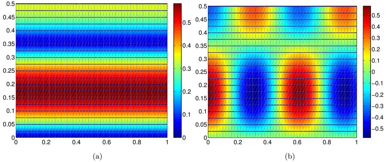
**Fig. 3.4.** Analytical results for the propagation at 800 Hz of the second mode of the first azimuthal order in a hard walled duct: (a) Absolute part of the acoustic pressure (b) Real part of the acoustic pressure.
