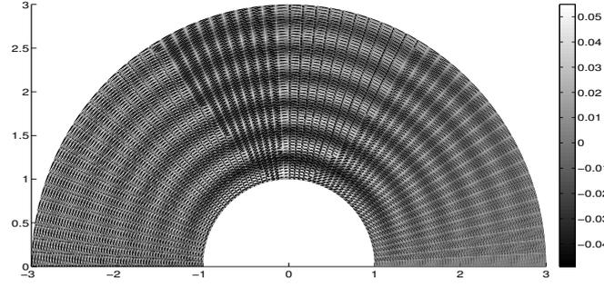
**Fig. 3.19.** Dipole radiation: real part of the computed pressure ( $1100Hz$ ,  $kr_S = 20.3$ ),  $r_S = 1m$ ,  $r_T = 3m$ , number of elements in the radial direction:  $n_r = 60$ , and in the circumferential one:  $n_\theta = 60$ , radial order of infinite elements  $m_0 = 2$ , circumferential order of infinite elements  $b_0 = 1$  and enrichment in the inner region  $V_{j1} = \{1\}$ : MIPUM 0 2 1.
