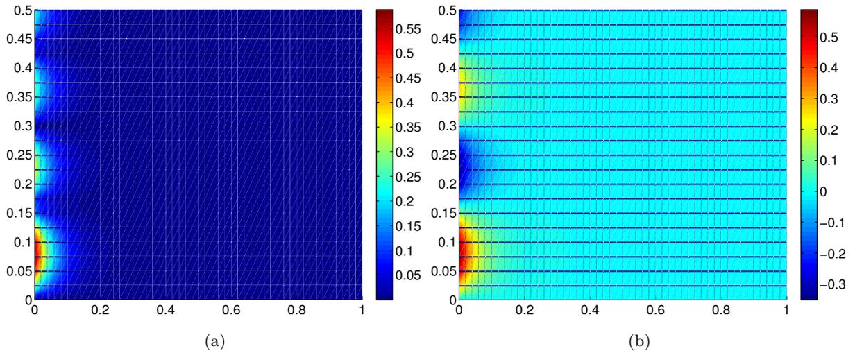
**Fig. 3.6.** MIPUM 0 computed results for the propagation at 800 Hz of the fourth mode of the first azimuthal order in a hard walled duct: (a) Absolute part of the acoustic pressure (b) Real part of the acoustic pressure.
