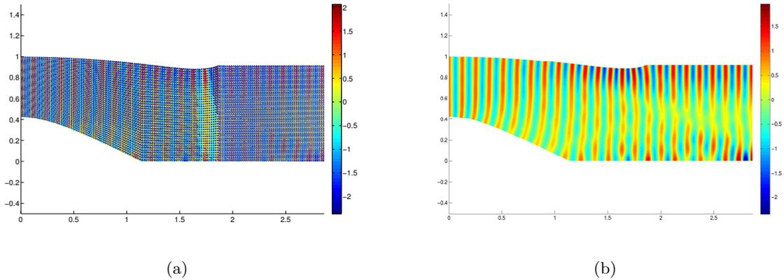
**Fig. 3.16.** Computed results (real part of the pressure) for plane wave propagation at  $1600\text{Hz}$  ( $ka = 29.57$  for  $a = 1\text{m}$ ): (a) Second order enrichment for the Partition of Unity Method (41226 dofs) (b) Linear Finite Element Method (42692 dofs).
