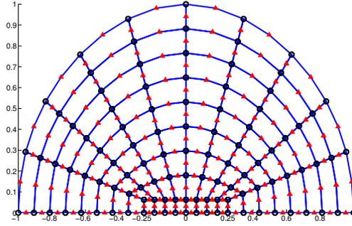
**Fig. 3.25.** Infinitesimal cylinder radiation: Mesh in the inner region ( $n_p = 8, n_r = 8$ ). Elements are in blue, nodes are black circles and mapping points are red triangles. The cylinder is on the range  $[-0.25, 0.25]$ .
