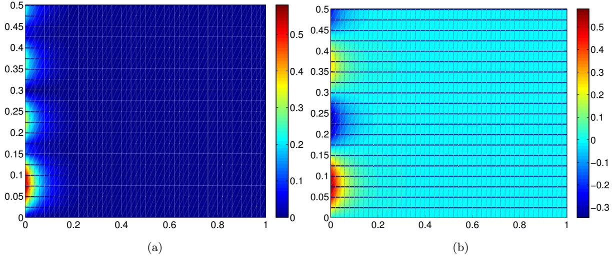
**Fig. 3.7.** Analytical results for the propagation at 800 Hz of the fourth mode of the first azimuthal order in a hard walled duct: (a) Absolute part of the acoustic pressure (b) Real part of the acoustic pressure.
