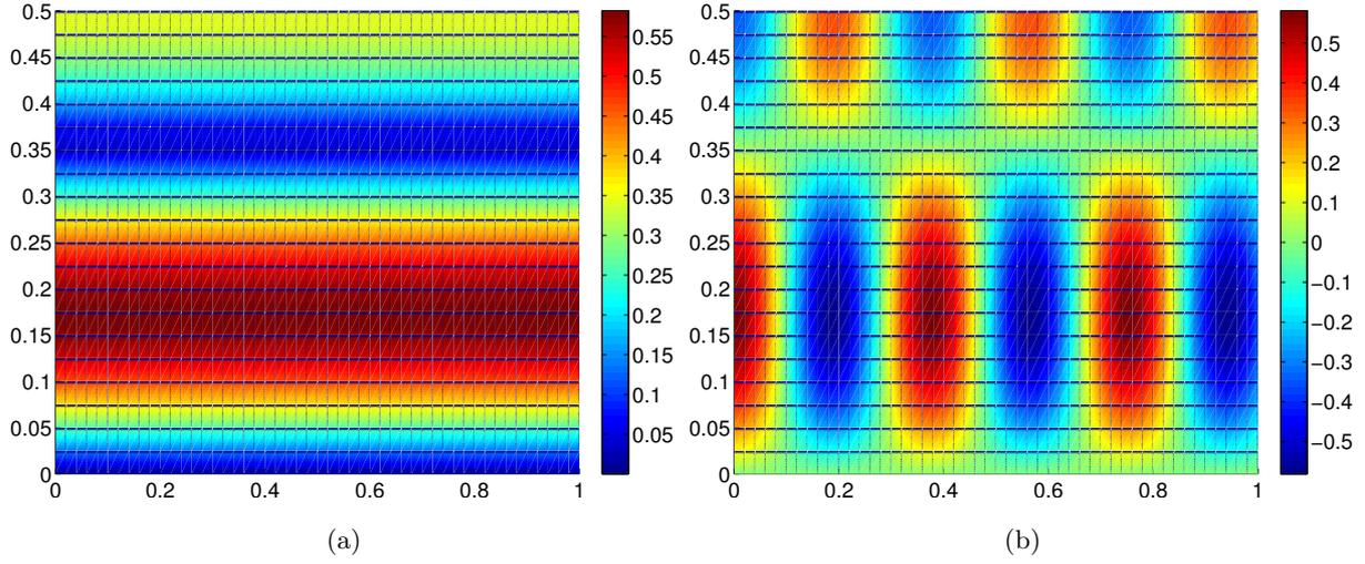
**Fig. 3.11.** MIPUM 0 computed results for the convected ( $\mathbf{v}_0 = -100m/s\mathbf{1}_z$ ) propagation at 800 Hz of the second mode of the first azimuthal order in a hard walled duct: (a) Absolute part of the acoustic pressure (b) Real part of the acoustic pressure.
