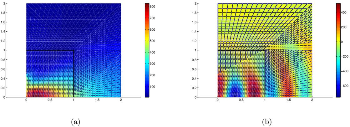
**Fig. 3.23.** MIPUM 0-4-1 computed results for the radiation of a rigid piston at 500 Hz. The black line represents the interface  $\Gamma$  separating the inner and outer region. (a) Absolute part of the acoustic pressure (b) Real part of the acoustic pressure.
