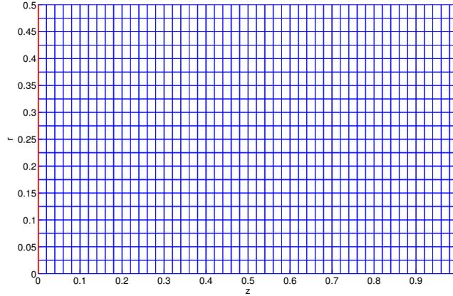
**Fig. 3.2.** Computational domain meshed with 50 elements in the axial direction and 20 in the radial one. The modal and transmitted boundary conditions are illustrated in red.
