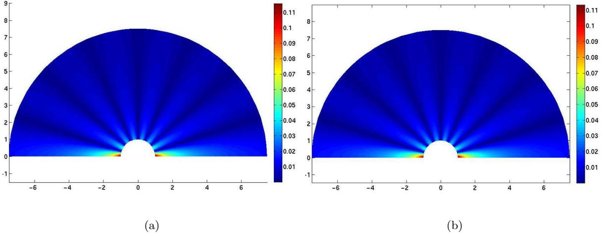
**Fig. 3.21.** Multipole ( $N = 7$ ) radiation: Absolute part of the MIPUM 0 2 1 computed (a) and analytic (b) pressure ( $700\text{Hz}$ ,  $kr_S = 12.94$ ), number of elements in the radial direction:  $n_r = 70$ , and in the circumferential one:  $n_\theta = 70$ .
