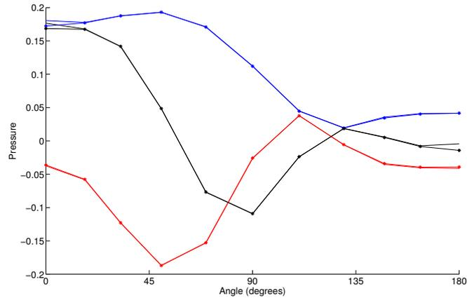
**Fig. 3.29.** Infinitesimal cylinder radiation with a third order enrichment at 500 Hz with a uniform mean flow  $\mathbf{v}_0 = -85m/s \mathbf{1}z$ ,  $n_p = 8$ ,  $n_r = 8$ : illustration of the analytical and the computed pressure along the interface  $\Gamma$ : absolute (blue), real (red) and imaginary (black) part of the pressure.
