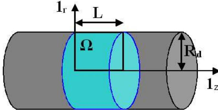
**Fig. 3.1.** Geometry of the duct: infinite duct in grey, finite duct in blue and the axisymmetric computational domain  $\Omega$  given by the black rectangular domain.
