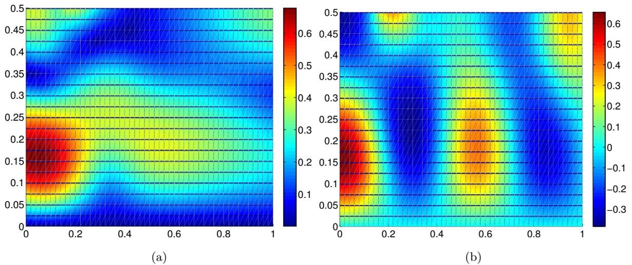
**Fig. 3.9.** MIPUM 0 computed results for the propagation at 800 Hz of the second mode of the first azimuthal order in a partially lined duct: (a) Absolute part of the acoustic pressure (b) Real part of the acoustic pressure.
