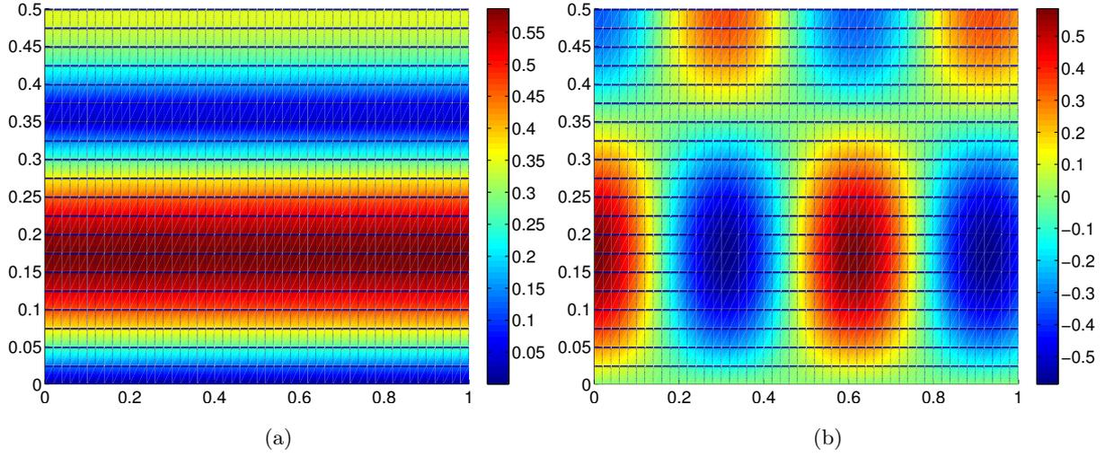
**Fig. 3.3.** MIPUM 0 computed results for the propagation at 800 Hz of the second mode of the first azimuthal order in a hard walled duct: (a) Absolute part of the acoustic pressure (b) Real part of the acoustic pressure.
