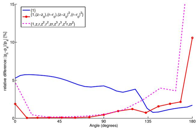
**Fig. 3.30.** Infinitesimal cylinder radiation at 500 Hz with a uniform mean flow  $\mathbf{v}_0 = -85\text{m/s } \mathbf{1z}$ : illustration of the relative difference [%] along the interface  $\Gamma$ . (Some simplifications have been made in the legend. The third order terms  $\{x, y, \dots\}$  have to be read as  $\{(x - x_0), (y - y_0), \dots\}$ )
