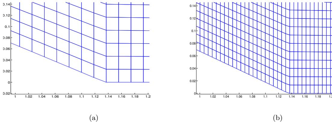
**Fig. 3.17.** Mesh around the spinner: (a) mesh  $200 \times 40$  (b) mesh  $600 \times 70$ .
