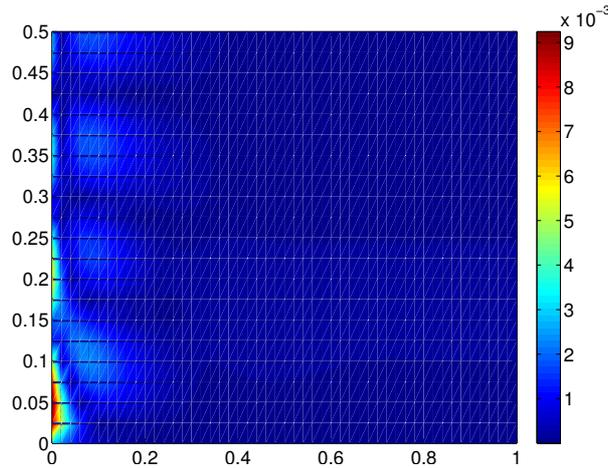
**Fig. 3.8.** Propagation at 800 Hz of the fourth mode of the first azimuthal order in a hard walled duct: MIPUM 0 discrete  $L^2$  norm.
