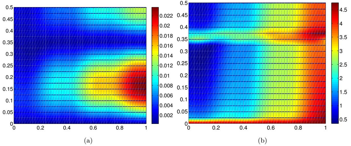
**Fig. 3.5.** Propagation at 800 Hz of the second mode of the first azimuthal order in a hard walled duct: MIPUM 0 (a) Discrete  $L^2$  norm (b) Relative discrete  $L^2$  norm [%].
