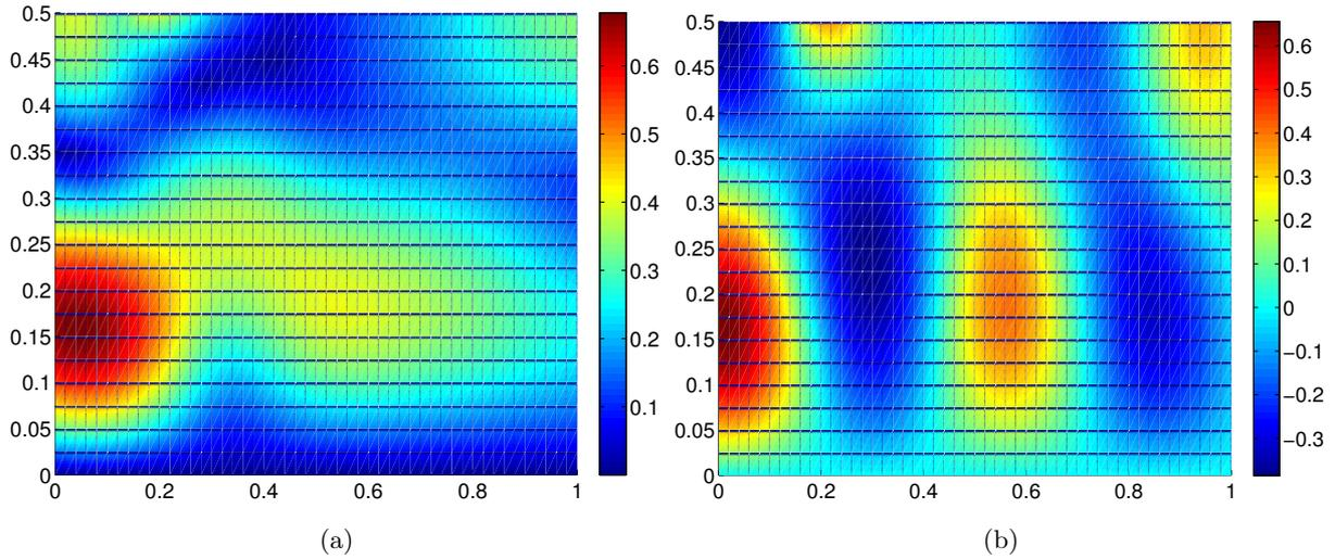
**Fig. 3.10.** Computed results with ACTRAN<sup>TM</sup> for the propagation at 800 Hz of the second mode of the first azimuthal order in a partially lined duct: (a) Absolute part of the acoustic pressure (b) Real part of the acoustic pressure.
