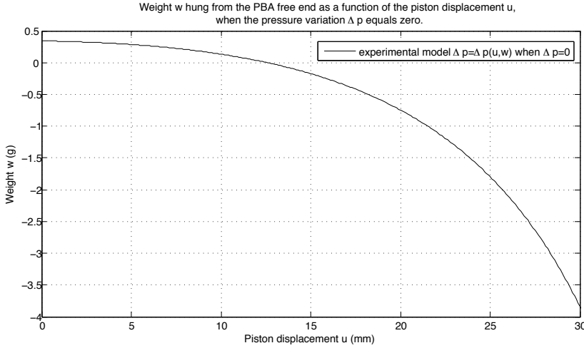
Figure 5.13: Weight w hung from the PBA free end as a function of the piston displacement u , when the pressure variation \Delta p equals zero. The solid line is the experimental model \Delta p = \Delta p(u, w) for \Delta p = 0 . In practice, when there is no pressure variation, it means that the PBA is not loaded but the experimental model forecasts a non-zero weight, apart from one value of u . u does not range above 30 mm because above this value the experimental model keeps on forecasting negative weights and even weights having an imaginary part.
