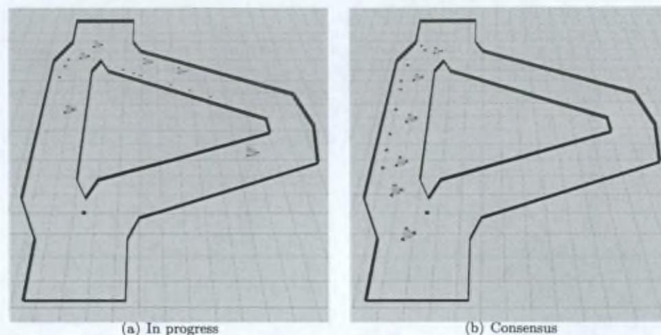
Figure 5.9: Shortest path selection process. Figure (a) shows a swarm of robots in the process of transporting objects from the starting point to the target location. Note that the robots use both branches of the environment. Figure (b) shows the state of the environment when the swarm of robots has reached consensus. The path selected by the swarm of robots is the shortest one.
