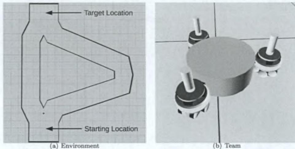
Figure 5.7: Task Scenario. The arena is a bridge-like environment with two branches of different lengths (see Figure (a)). Teams of robots carry objects (see Figure (b)) from one end of the arena to the other. Robots must choose to take either the left or the right path.
