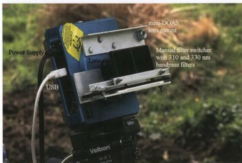
Figure 6.5 The camera deployed in the field, showing its different components. (Sunshade was taken off for the photograph)
