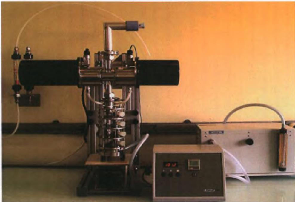
Figure 41. Spraytec<sup>®</sup> device connected to a multi-stage liquid impinger (Pilcer, 2008a)
