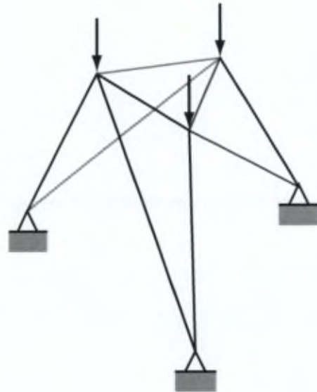
Figure 5.10: 9 bar 3D structure
