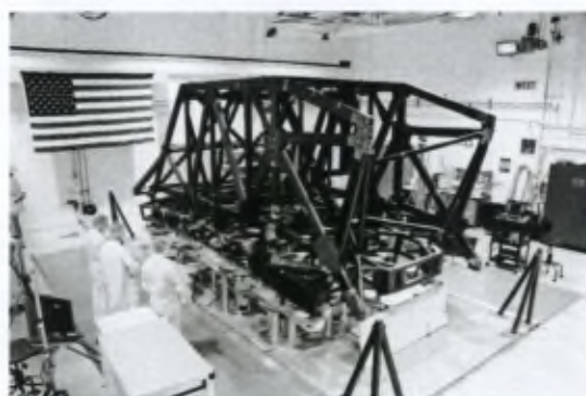
Figure 2.2: The backplane support structure for NASA's James Webb Space Telescope in Magna, Utah. Image courtesy of NASA
