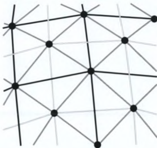
Figure 3.3: A configuration of three grids of varying orientation with common nodes
