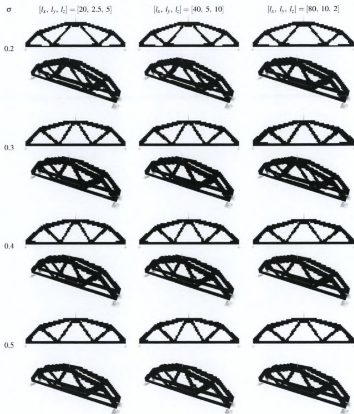
Figure 6.7: 3D bridge problem. Resulting topologies for various values of the standard deviation \sigma and the correlation length l
