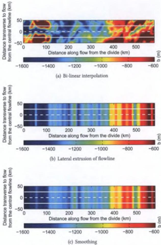
Figure 6.5: Bedrock elevation  $b$  of the domain in plane view obtained by (a) bi-linear interpolation of the data (Exp. 1), (b) lateral extrusion of central flowline data (Exp. 2), and (c) smoothing of bedrock elevation over 25 km (Exp. 3) ( $\Delta x = 1$  km). The central flowline is shown as a dashed white line. The domain lateral boundaries corresponding to widths  $\omega = 50$  km and  $\omega = 100$  km are shown as solid white lines and lateral borders of the figure respectively.
