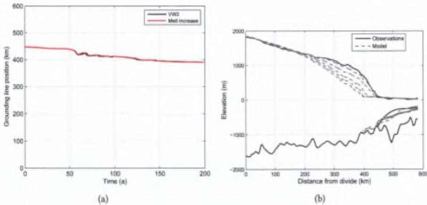
**Figure 5.11:** Thwaites Glacier (a) grounding-line position as a function of time for Exps. VW3 and basal melt increase ( $+ 5 \text{ m a}^{-1}$ ) and (b) modeled geometry profiles for the basal melt increase experiment after 10, 50, 100, 150 and 200 years (from right to left). The observed geometry profile is also shown.
