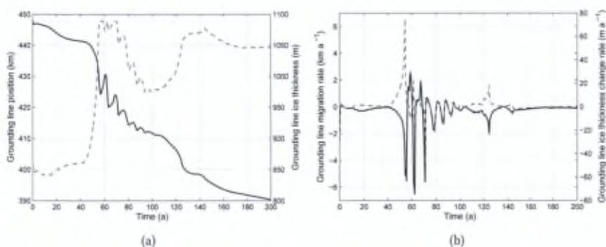
**Figure 5.6:** Results of Exp. VW3: (a) grounding-line position (solid black line) and ice thickness (dashed gray line); (b) grounding-line migration rate (solid black line) and ice-thickness change rate (dashed gray line).
