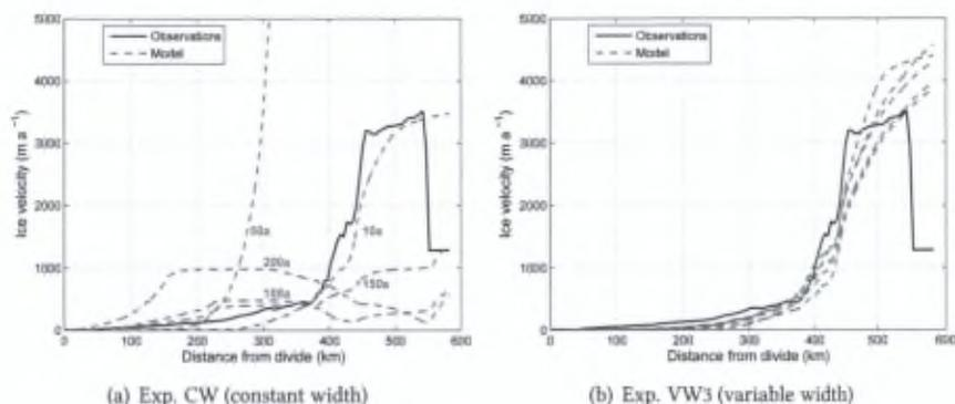
**Figure 5.5:** Modeled velocity profiles of Thwaites Glacier after 10, 50, 100, 150 and 200 years (labeled for (a) Exp. CW and from left to right for (b) Exp. VW3). The velocity profile of (a) is truncated at  $5000 \text{ m a}^{-1}$  to be compared to (b).
