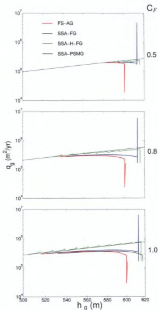
Figure 3.5: GL ice flux  $q_g$  as a function of GL ice thickness  $h_g$  for the four models and for the three different buttressing values, compared with the Schoof [2007a] solution (in grey).
