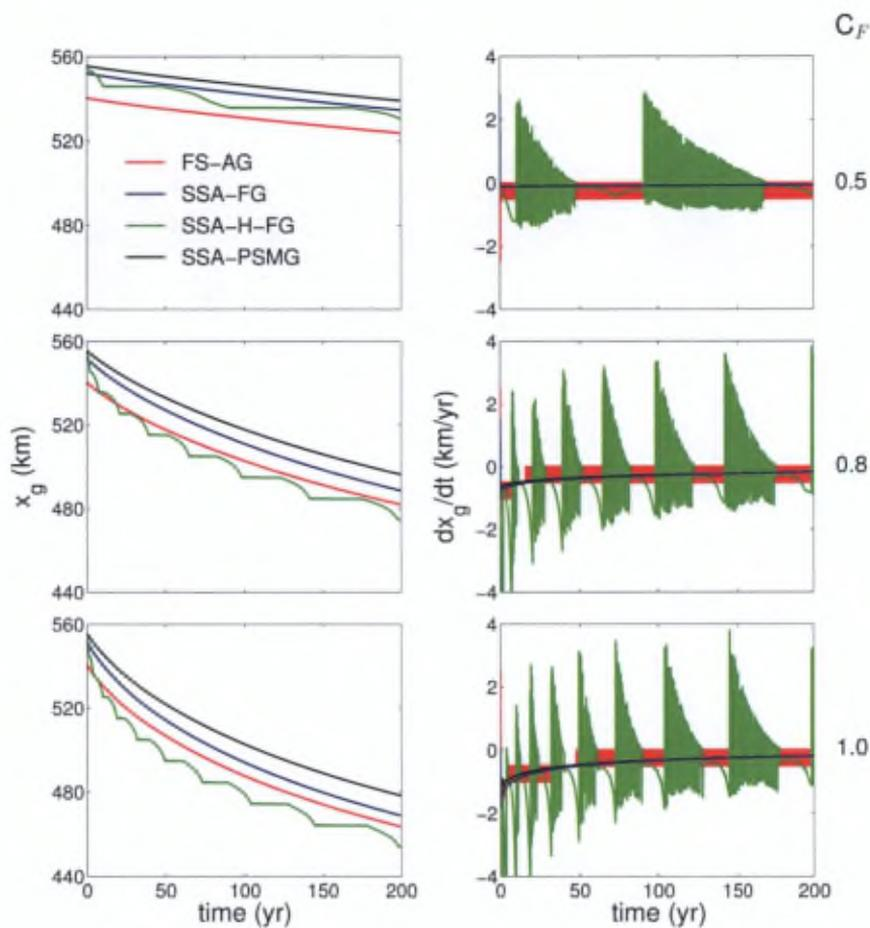
**Figure 3.2:** Grounding-line position  $x_g$  (left) and migration rate  $dx_g/dt$  (right) as a function of time for the four models and for the three buttressing values ( $C_F = 0.5$  on the first line,  $C_F = 0.8$  on the second line and  $C_F = 1$  on the third line).
