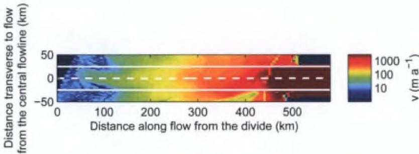
Figure 6.4: Observed ice velocity  $v$  of the domain in plane view obtained by bi-linear interpolation of the data ( $\Delta x = 1$  km). The central flowline is shown as a dashed white line. The domain lateral boundaries corresponding to widths  $\omega = 50$  km and  $\omega = 100$  km are shown as solid white lines and lateral borders of the figure respectively.
