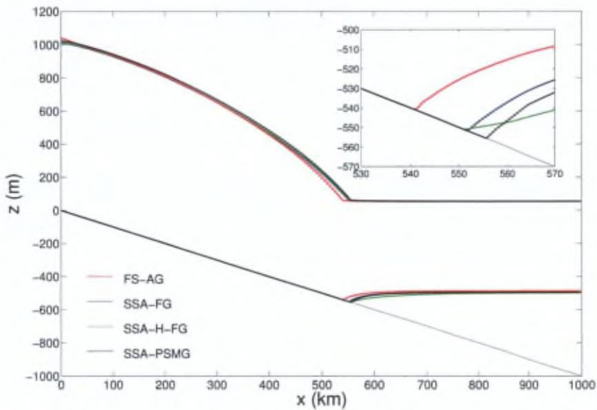
**Figure 3.1:** Initial steady-state geometry ( $C_F = 0.4$ ) for all models. The inset emphasizes the differences in GL position. SSA-H-FG lower surface has a quite different shape with respect to the three other models due to its coarser resolution (10 km).
