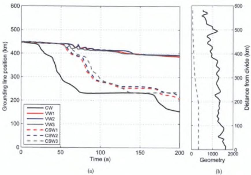
**Figure 5.7:** (a) Thwaites grounding-line position as a function of time for the width experiments. (b) Bedrock depth and VW3 width.
