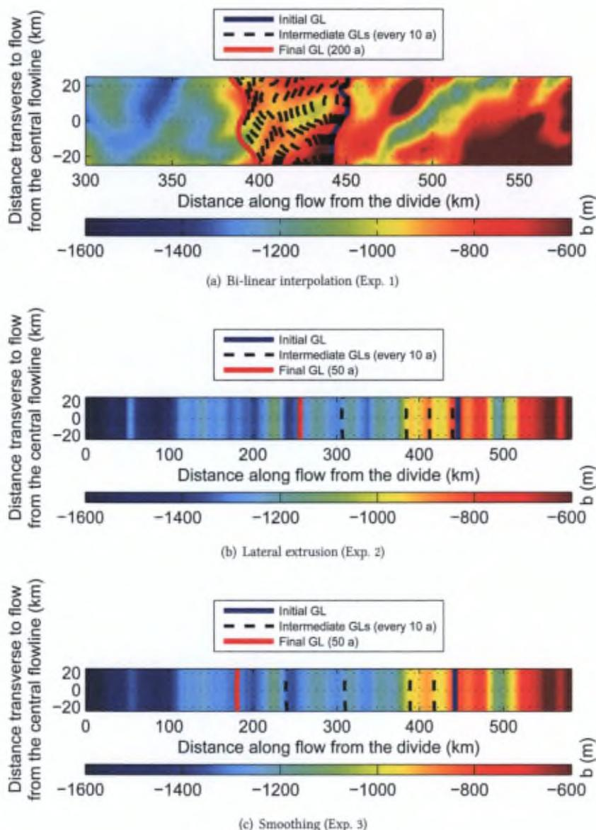
Figure 6.8: Grounding-line (GL) positions in plane view plotted every 10 year with the corresponding bedrock elevation  $b$  for three simulations: (a) bi-linear interpolation of the data (Exp. 1), (b) lateral extrusion of central flowline data (Exp. 2), and (c) smoothing of bedrock elevation over 25 km (Exp. 3) ( $\Delta x = 0.5$  km).
