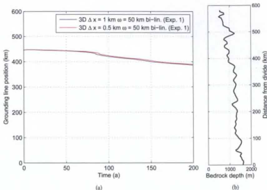
**Figure 6.7:** (a) Thwaites central grounding-line position as a function of time (200 a) for Exp. 1 (bi-linear interpolation of data) with  $\Delta x = 0.5$  and  $1 \text{ km}$  and  $\omega = 50 \text{ km}$ . (b) Bedrock depth.
