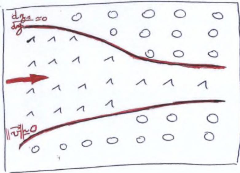
**Figure 6.14:** Schematic plane-view representation of the method used to incorporate Thwaites Glacier drainage basin into the model. The limits of the drainage basin (in red) are defined by surface elevation slope  $\frac{dz_s}{dy} \approx 0$  and ice velocity vector  $v \approx 0$ . A value of 1 is assigned to pixels within the drainage basin and a value of 0 outside the basin. The ice flow direction is represented by the red arrow.
