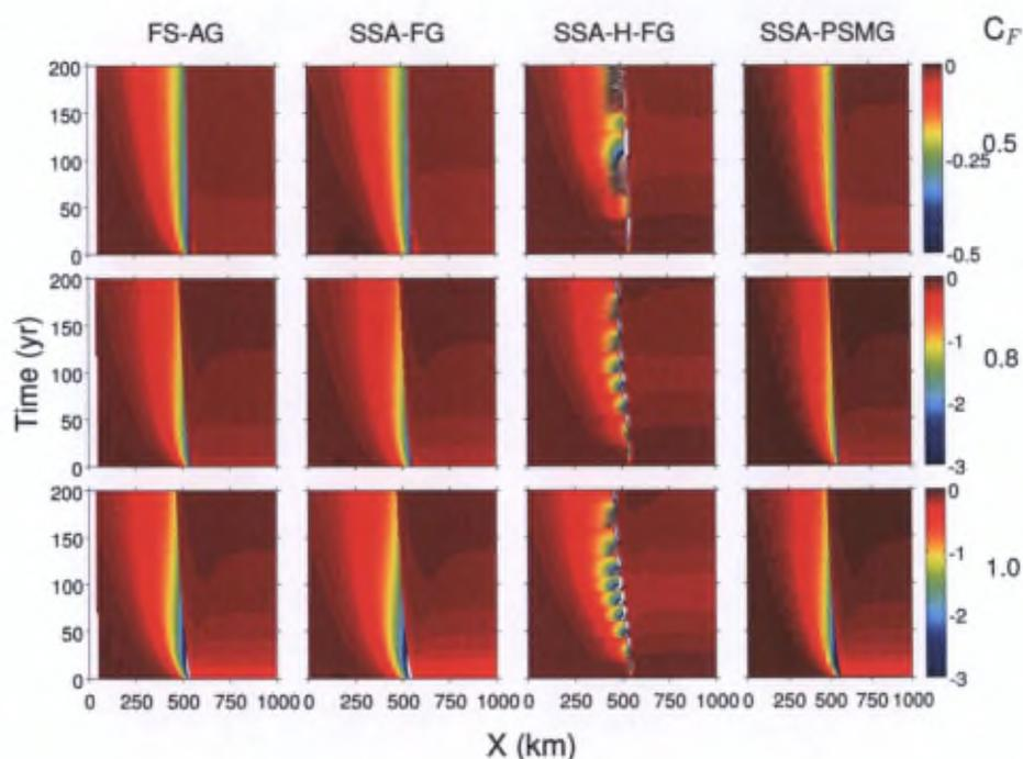
Figure 3.3: Rate of surface elevation change ( $m\ yr^{-1}$ ) as a function of time and horizontal distance ( $x = 0$  corresponds to the ice divide and  $x_f = 1000\ km$  is the calving front) for the three buttressing values (lines) and for the four models (columns).
