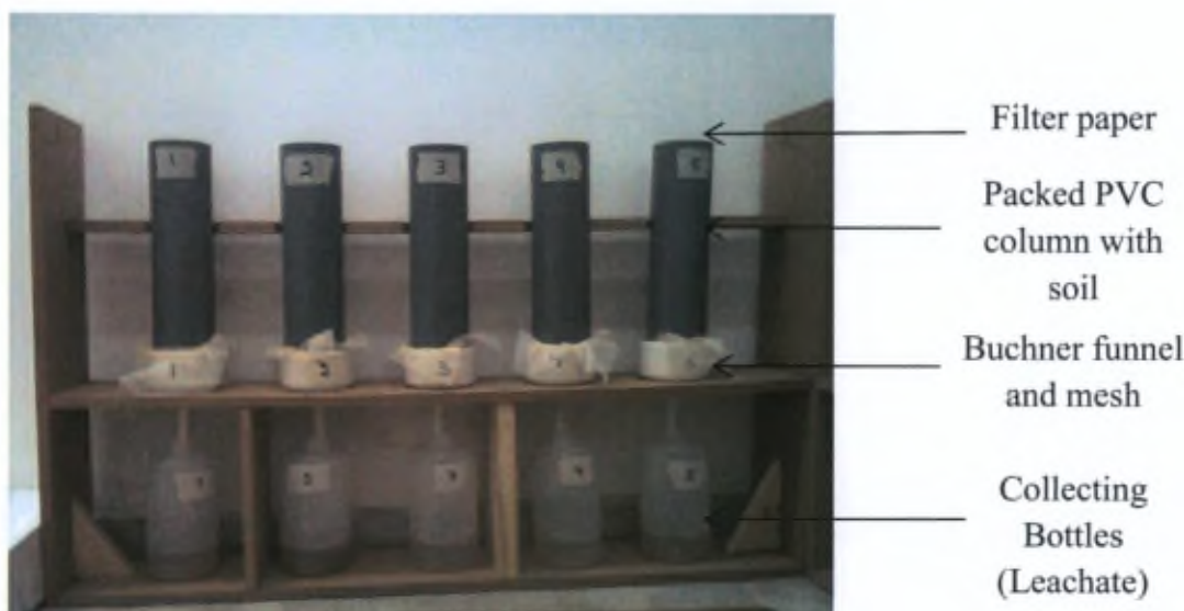
Figure 2.8: Leaching columns system.
