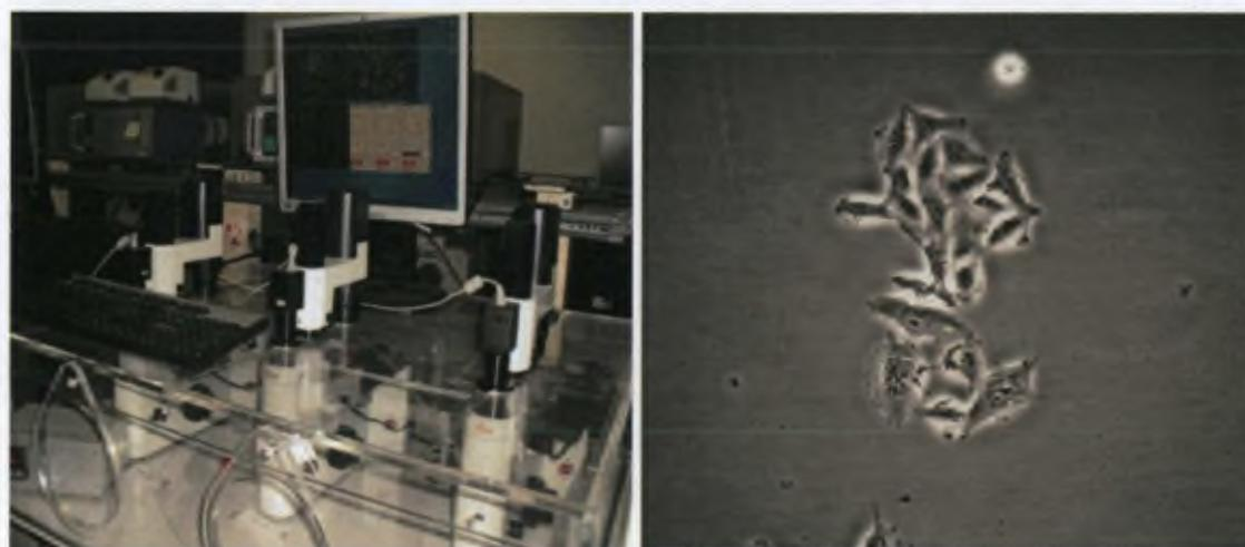
Figure 6.3 – Left: The device used for computer-assisted videomicroscopy. Right: Illustration of cells seen in the microscope's field of view (A594 NSCLC cell line).
