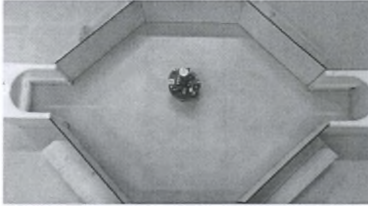
Figure 5.8: Snapshot recorded during the first TAM reliability experiment, where a single e-puck robot has to continuously perform two stationary atomic tasks. In the situation shown, the e-puck has recently completed the blue task represented by the TAM on the right side. The TAM on the left side is now announcing a green task, which is perceived by the e-puck.
