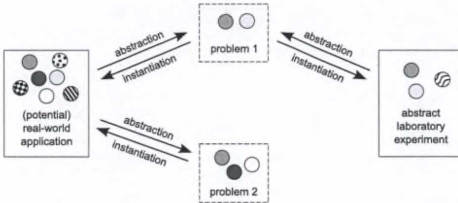
Figure 2.1: Illustration of the process of abstraction as employed in swarm robotics research. Problem instances and abstract problems are represented as boxes with full and dashed borders, respectively. Instances and problems alike possess various aspects, represented as small circles with different colors/patterns. Abstract problems possess only aspects essential to them. Instances such as real-world applications typically possess inessential aspects in addition to the essential aspects of the abstract problems they instantiate. Laboratory experiments are abstract instances in the sense that they typically possess all the essential and only few inessential aspects.
