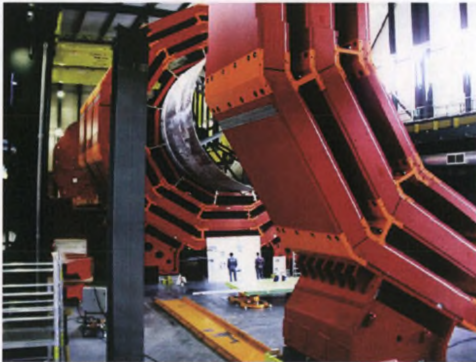
Figure 12: View of the yoke elements around the solenoid [9].
