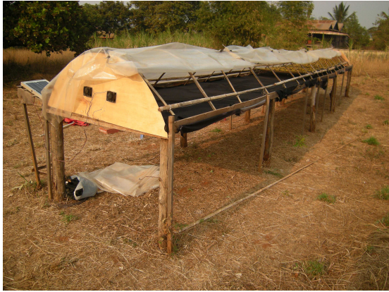
Fig. 3. Tunnel solar dryer built in Banlung.
