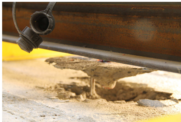
Figure 12. Pull-Out test: concrete cone at ultimate load
