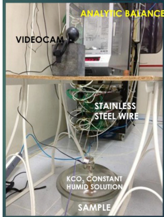
Figure 3. Experimental setup for the measurement of the diffusion coefficient of kapton/water and GEM/water systems.
